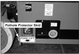
Figure 8.12—Pothole Protector Skid
