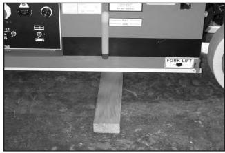
Figure 8.13—Pothole Protector Interlock Test
