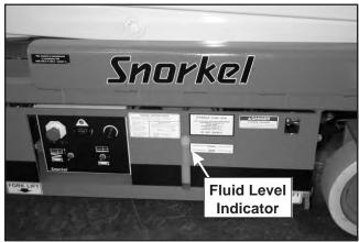
Figure 8.6—Fluid Level Indicator
